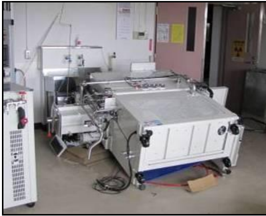
Topped unrestrained lab workstations (2011 M9.0 Japan earthquake)
